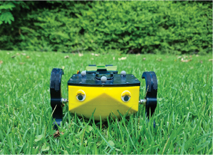
▲ The AmphiSAW, with its paddle-like leg attachments for land mobility. (Photo credit: Dr. David Zarrouk/BGU)
